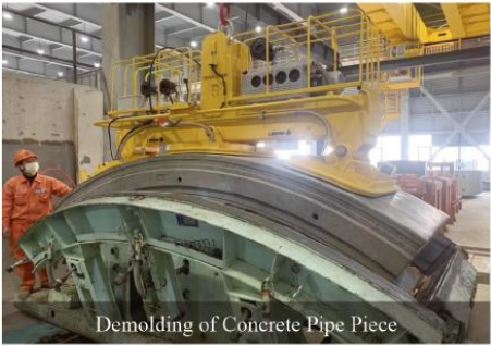
Demolding of Concrete Pipe Piece AC-Vacuum Lifter (3 Suckers) HP-M5000-3S (5000KG)
