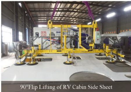
90°Flip Lifting of RV Cabin Side Sheet AC-Vacuum Lifter (10 Suckers) HP-WDF500-10S (500KG)
