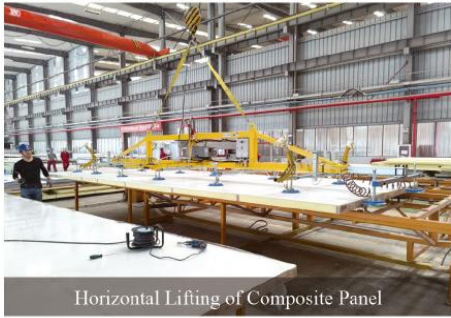
Horizontal Lifting of Composite Panel AC-Vacuum Lifter (14 Suckers) HP-WBSJ1500-14S (1500KG)
