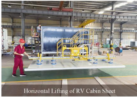
Horizontal Lifting of RV Cabin Sheet DC-Vacuum Lifter (8 Suckers) HP-WBSZ200-8S (200KG)
